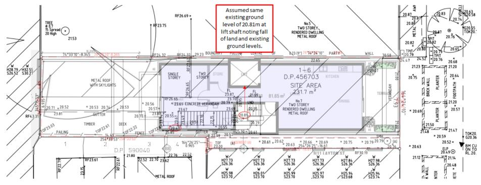
Figure 1 - Overlay of level 5 plan over survey plan with existing ground levels shown. Source: CPS edit of architectural and survey plans
